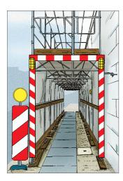
Risks to pedestrians from on-site traffic can be reduced by providing segregated pedestrian and vehicular routes that are properly demarcated and by providing added protection for pedestrians at places of particular risk. Crossing points require particular attention.
